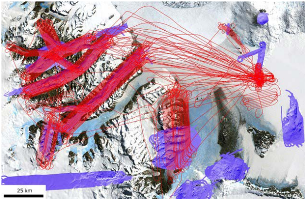
Figure 4. Flight lines for the new 2014–2015 survey (shown in red) over the extent of the 2001 survey (shown in purple) digital elevation model hillshades. Base map is the Landsat Image Mosaic of Antarctica (Bindschadler et al., 2008).
